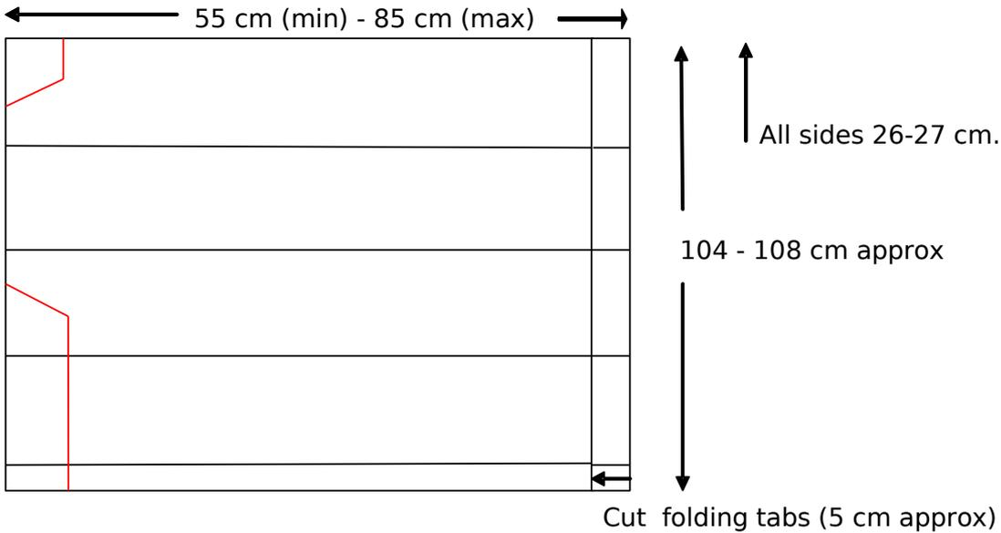
Size: Between 2ft (60cm) and 2.5 ft (66cm) in length and 10-11 inches (26-28cm) in width. Mark lines with a pen for the front sloping angles (indicated in red). \* It's easier to mark and cut the front shape in 3D, once the box is assembled and you can see the intended shape.
